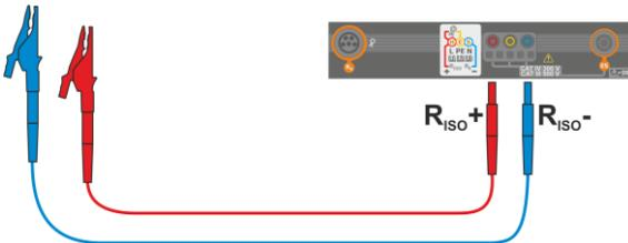
Connect the probes to the meter.
