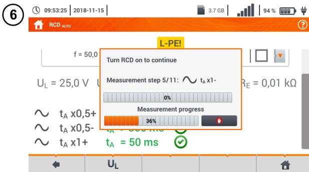
Tested RCD switch, must be **turned on** after each triggering, measurements are **completed**.
