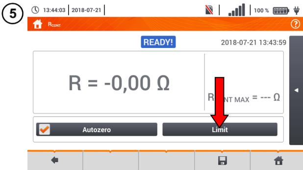
Set the acceptable limit resistance of the measured object.
