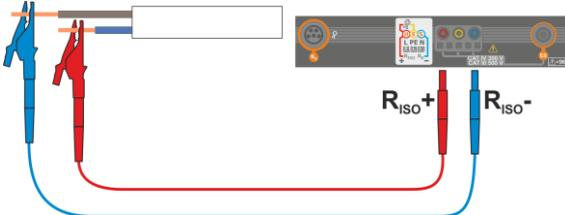
Connect test leads according to the drawing.
