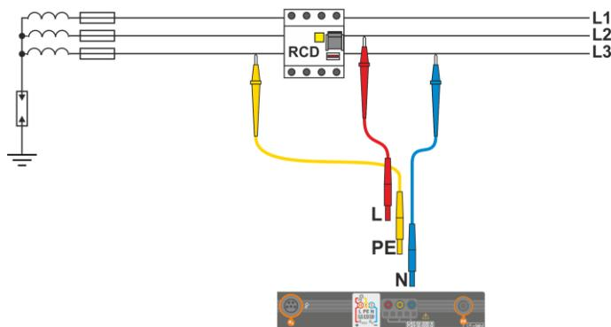
**Fig. 3.9** RCD testing without the PE conductor
