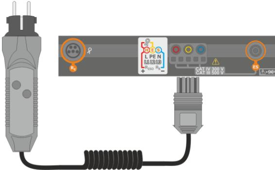
Connect **WS-03 adapter** or **WS-04 adapter** with UNI-Schuko outlet plug.
