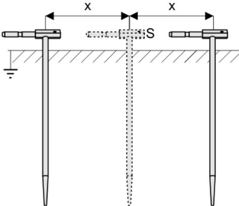
Repeat the steps **(2)(5)(6)** for two additional locations of the voltage electrode **S**:
