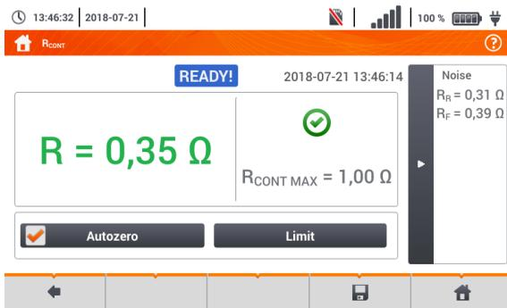
$R_F$  – result obtained for a **positive** polarity of the measuring current
