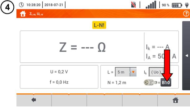
The result can be compared against the acceptable fault loop impedance  $Z_{sdop}$ , determined on the basis of the fuse parameters of the tested circuit:
