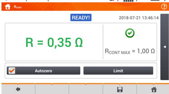
The result is the arithmetic mean of the values of two measurements at a current of 200 mA with opposite polarities  $R_F$  and  $R_R$ .
