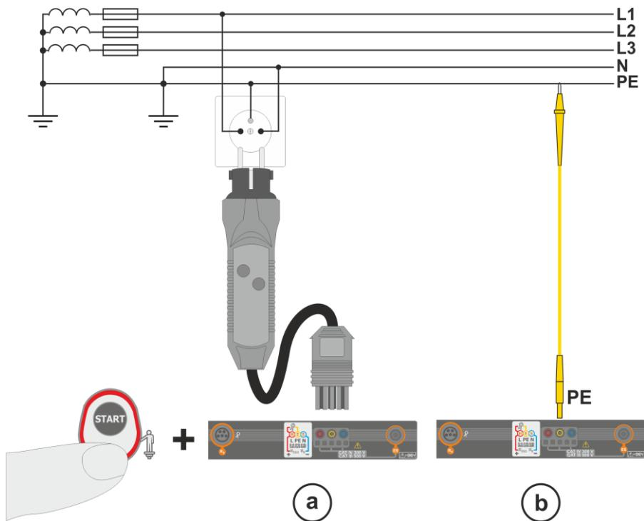
When the meter is connected as in the drawing, touch the contact electrode and wait for about **1 second**. If voltage is detected on the PE conductor, the device:
