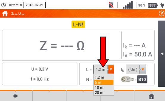
The correctness of the measurement depends on the correct adjustment of the length of leads.
