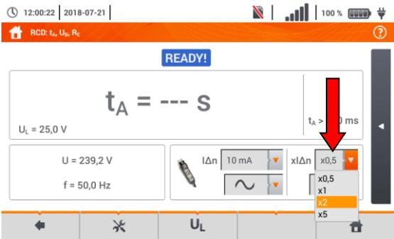
If the RCD  $t_A$  mode has been selected in step ①, set the forced current in the RCD test.
