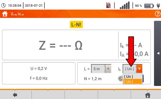
The prospective short-circuit current  $I_k$  can be calculated based on one of two values:
