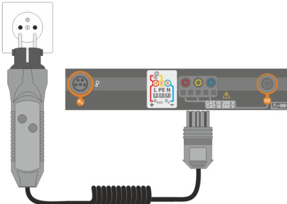
Connect the adapter to the test socket.
