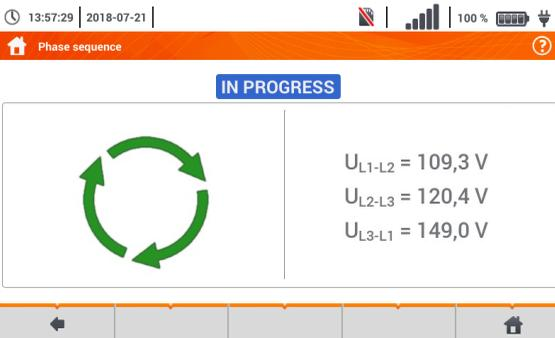
The phase sequence is **correct**, i.e. the phase sequence is in **clockwise** direction.
