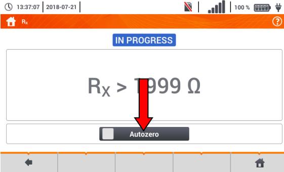
Select **Autozero** to eliminate the resistance of test leads.
