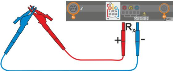
To **disable compensation** of the resistance of leads, repeat steps ②③④ with **open** test leads. Then the measurement result will **contain the resistance of test leads**.
