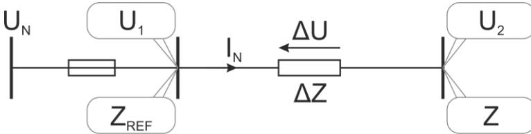
The voltage drop is calculated according to the following formula:
