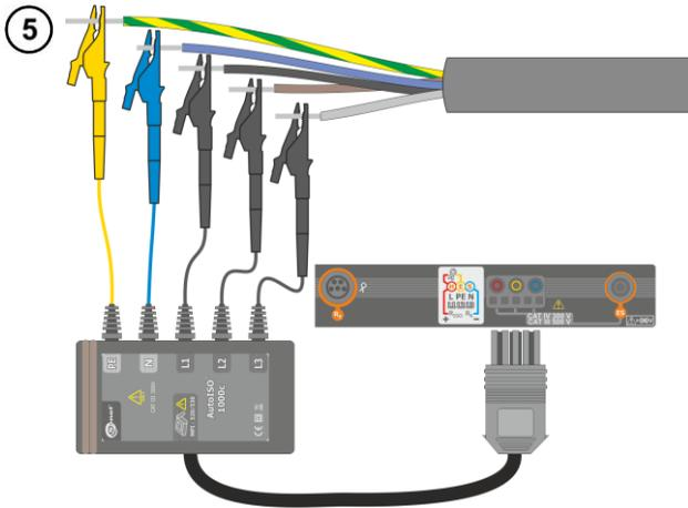
Connect AutolSO-1000c adapter to the lead tested.
