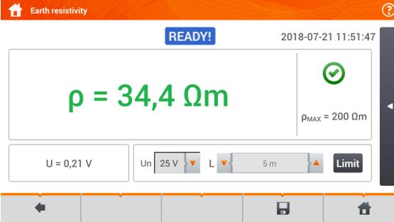
Signal lights for reaching the limit (section 3.7.1 step 4):
