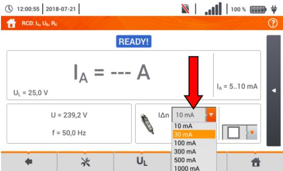
The correctness of the assessment of the test circuit breaker efficiency is dependent on the rated residual current.
