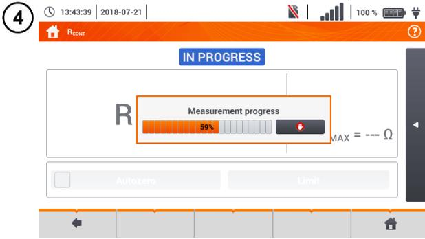
To **disable compensation** of the resistance of leads, repeat steps ② ③ with **open** test leads. Then the measurement result will **contain the resistance of test leads**.
