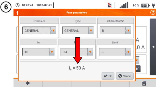
The current is calculated after setting parameters in steps (6) (7).  $I_a$  – current ensuring automatic triggering of a protective device within a required time.
