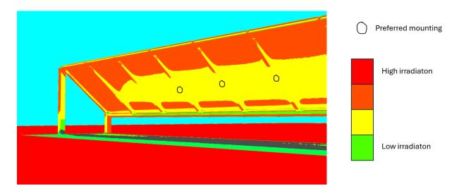
In case of different configurations of PV modules in a PV string the PV reference cell must be placed in the centre of the PV string. Some of the recommended placements of the reference cell are shown in the figure bellow with the black circles.
