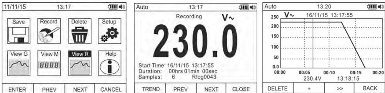
Fig. 20: Recalling recordings to the display
