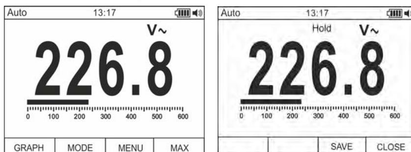
Fig. 4: Saving the value frozen on the display
