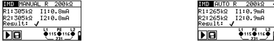
Figure 5.17: Examples of IMD test results
