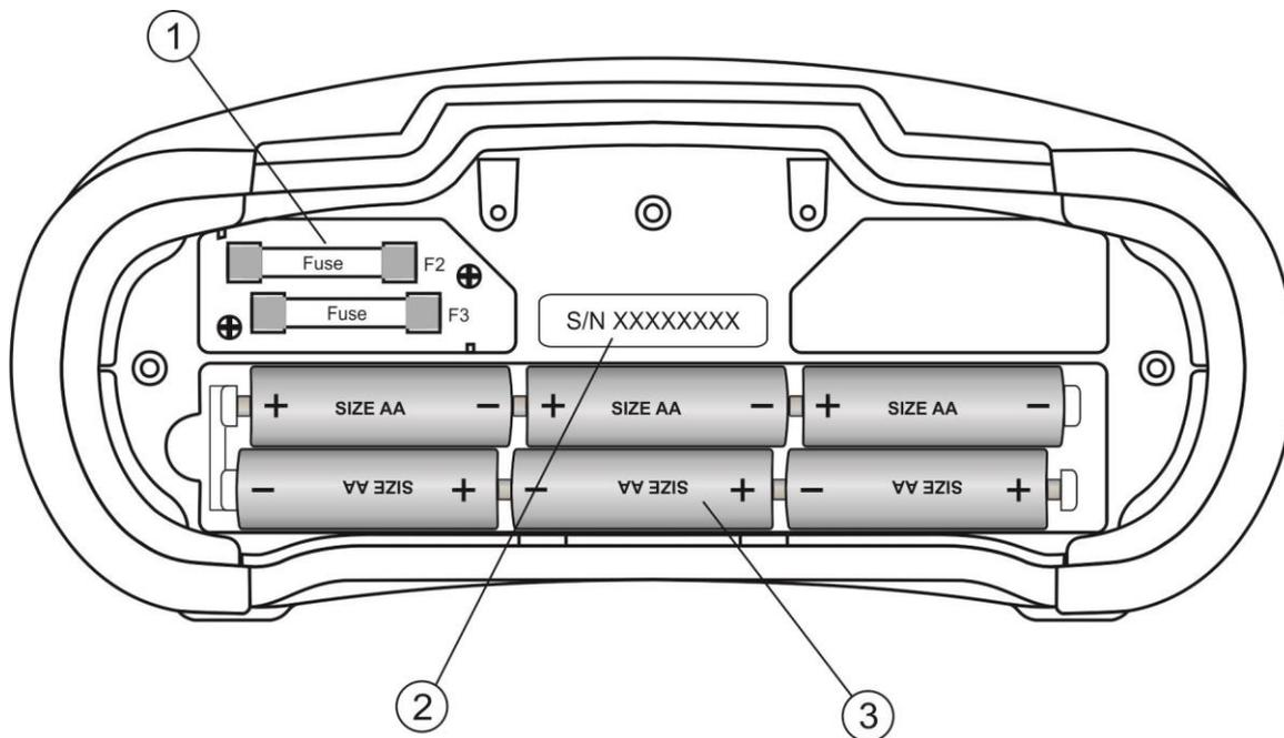
Figure 3.4: Battery and fuse compartment
