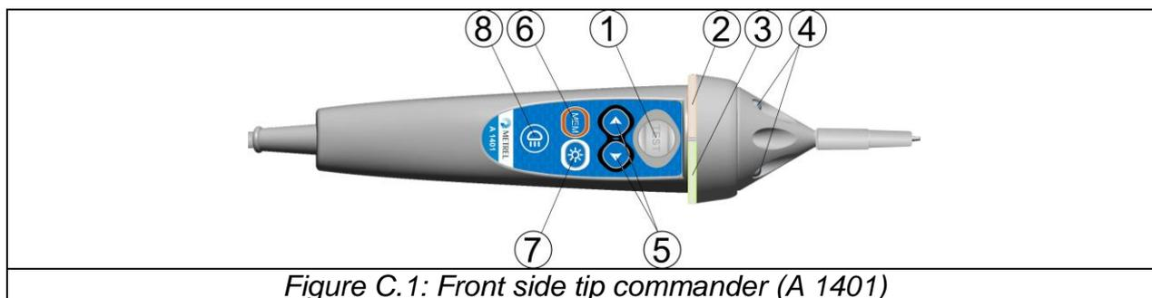
Figure C.1: Front side tip commander (A 1401)
