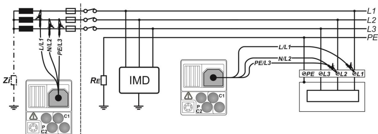
Figure 5.9: Voltage drop measurement in IT system – connection of 3-wire test lead
