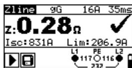
Figure 5.8: Example of line impedance measurement result
