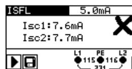
Figure 5.14: Examples of measurement results for the first fault leakage current
