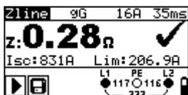
Figure 4.1: Typical function display
