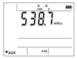
Then convert the voltage displayed into a current using the transformation ratio (TR) of the sensor:
