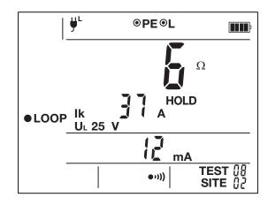
■ The measurement starts automatically. The result is displayed: the loop impedance and the short-circuit current (lk). Press the **TEST** key to return to voltage measurement.
